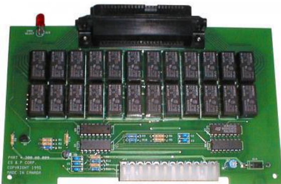
Model RY912 12-Line Relay Board For use with TE903NP or TE904NP Master Stations or with DPH100W Concierge Phone
