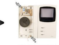
Remove screws b, in order to take off the bottom part of the handset.
