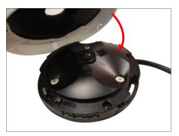
2. Twist the dome cover towards the right to lock the cover into place.
