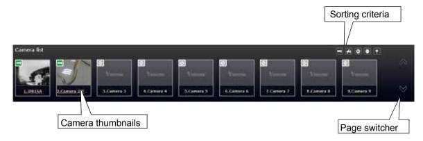
Depending on the size and screen resolution of your monitor, the snapshots of 8 cameras are displayed in this panel. If a user logged in using a credential of a limited access, he may only see cameras that he can access instead of all of the cameras.
