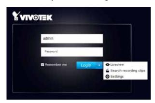
The NVR system features a simple UI structure which consists of a Liveview window, a Playback utility, and a system Settings window. Once logged in, you can move from one window to another by selecting the hot link buttons on the upper right of the screen.
