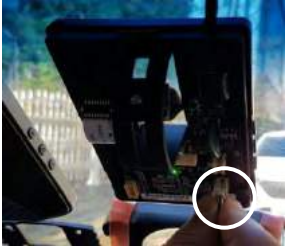
① Connect the configuration cable to the connector of main body
