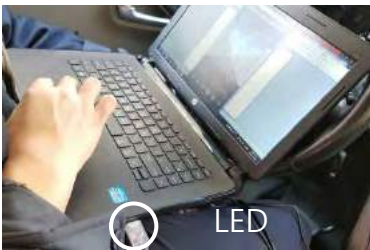
② Connect the configuration cable to your laptop PC , afterwards , run the manager program ,
