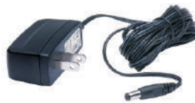
Power Supply Input: 100~240 VAC 50/60 Hz 1.2A Output: +24 VDC, 1.5A
