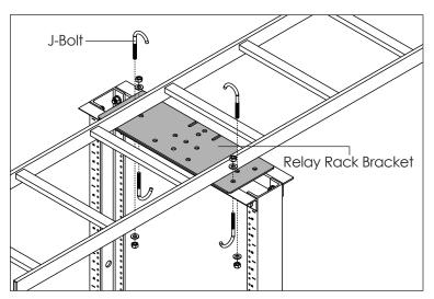
Option 2: Mount bracket perpendicular to rack as shown using 2 J-Bolts. Then mount ladder running perpendicular to rack as shown using 2 J-Bolts.
