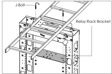
Option 2: Place ladder on top and bracket underneath perpendicular to rack as shown. Secure both of them using 2 J-Bolts.
