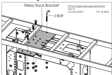
Option 1: Mount bracket parallel to rack as shown using 2 J-Bolts. Then mount ladder facing parallel to rack as shown using 2 J-Bolts.
