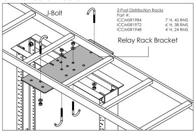
Option 1: Mount bracket parallel to rack as shown using 2 J-Bolts. Then mount ladder running parallel to rack as shown using 2 J-Bolts.
