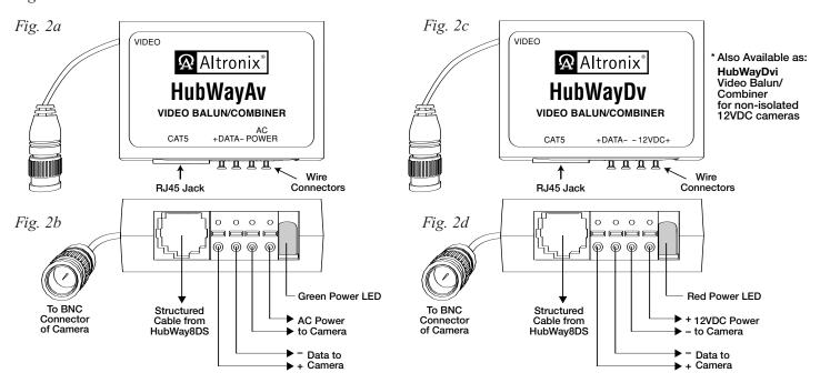
HubWayAv passes AC voltage from pins 4, 5, 7, 8 to terminals marked [AC Power] (Fig. 3, pg. 5).
