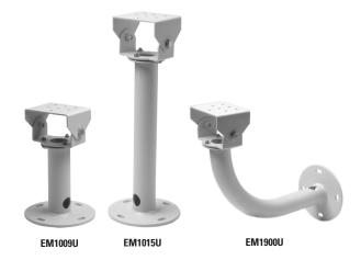
The **EM1009U/EM1015U/EM1900U** are medium duty enclosure mounts capable of supporting loads up to 40 lb (18.14 kg). Designed for ceiling/pedestal and wall applications, these versatile mounts can be used with Pelco enclosures having a 2-inch (5.08 cm) mounting hole pattern.
