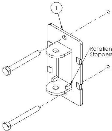
Step 3: Attaching the wall plate to the mounting surface (Lag Screws not included)
