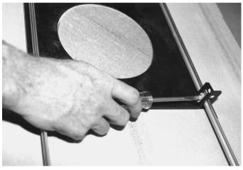
Figure 3.3 Tighten Bracket Securing Screw
