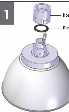
Remove housing coupling and gasket.
