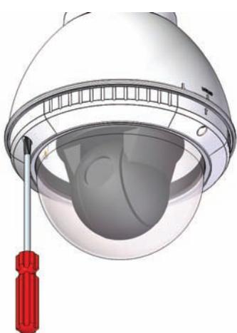
**Fasten down the dome with a Phillips screwdriver.**
