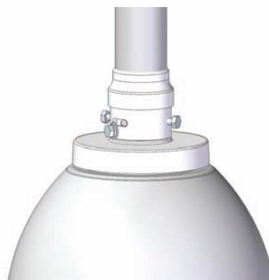
**Slide the grommet down over the coupling to prevent water from entering and complete the assembly go to block 18.**
