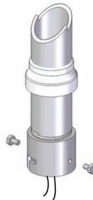
**Screw the (2) bolts into the coupling.**
