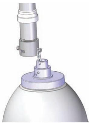
**Loop the lanyard over the set screw to temporarily hold housing.**
