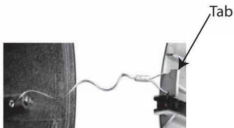
**Loop the lanyard around the tab inside the housing.**
