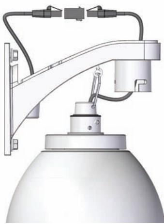
Feed wiring into wall mount,
