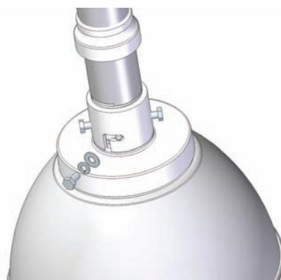
**Undo the lanyard, pull housing up and twist secure with the locking bolt and washers.**
