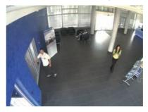
You can suppress this effect using software (e.g. in the browser) so that a new and appropriately corrected image can be displayed live. A side effect of this correction, however, is that a cushion shape appears around the edges of the image.
