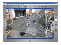
The panel at the bottom right-hand corner always displays the most recent event image of whatever camera is visible in the large panel. Double-click on a small camera panel to move this camera's live image to the large panel. Click the **Add cameras** button at any time to add MOBOTIX cameras to MxEasy (max. 16 cameras in total).
