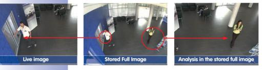
This means that you can use the vPTZ features in VGA resolution to pan, tilt and zoom the live image while the camera is e.g. recording full images at 1 fps in MEGA or QXGA resolution.
