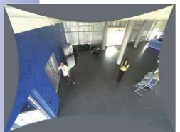
The image distortion caused by the L22 90° Wide Angle lens can be corrected (see Section 3.4). Since this function requires more computing power, it should not be enabled in the live image for applications that require a maximum frame rate. The image distortion in the recording can also be corrected at a later time.
