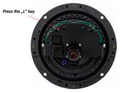
After about two more seconds, the camera is accessible via its factory IP address (see label on the camera housing).
