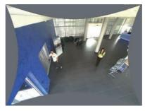
To hide this cushion effect, you simply have to zoom in on the image slightly. Although this reduces the size of the captured area, the image is almost distortion-free compared to the original.
