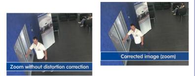
We recommend activating lens distortion correction, especially for applications with a low frame rate and non-zoomed images (e.g. when using the D24M as a webcam). However, images can usually be corrected at a later point in time when searching recorded images. This saves on processing power during recording and increases the frame rate. The more you zoom in on the image, the less distorted the image should appear.
