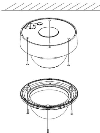
4. Remove the IR LED cover to adjust the lens and the viewing angle.
