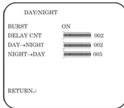
**Burst:** Enable/disable the color burst component of the video signal when the camera switches to B/W. ON mode maintains the same color signal in B/W so that the video signal provides better compatibility with certain color equipment. OFF mode removes the color burst signal B/W video and increase the total TV lines.
