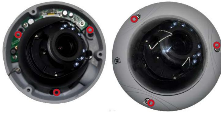
**Note:** Ensure that the screws highlighted above with a “○” have been tightened securely to prevent water seepage.
