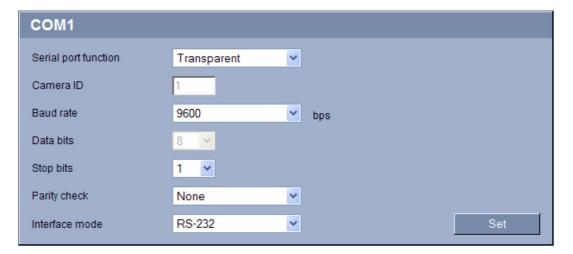
You can configure the serial interface parameters (orange terminal block) to meet your requirements.
