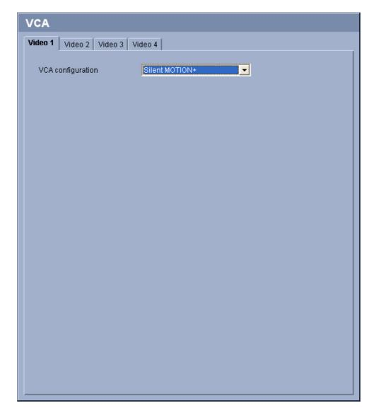
The VideoJet X40 contains an integrated video content analysis (VCA), which can detect and analyze changes in the signal on the basis of image processing. Such changes can be due to movements in the camera's field of view.
