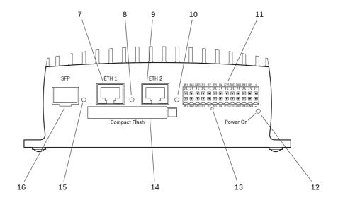
**7 ETH 1** RJ45 socket for connecting to an Ethernet LAN (local network), 10/100 MBit Base-T
