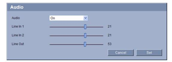
You can set the gain of the audio signals to suit your specific requirements. The current video image is shown in the small window next to the slide controls to help you check the selected audio source and improve assignments. Your changes are effective immediately.
