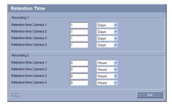
You can specify the retention times for recordings. If the available memory capacity of a medium has been used, older recordings are only overwritten if the retention time entered here has expired.
