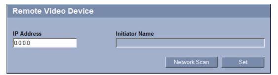
You can allow a remote video device to use the VideoJet X40 storage media. This means you can record video images from a camera that does not have its own storage media, for example. Once you have entered the IP address of the remote video device and saved it by pressing **Set**, the VideoJet X40 is then displayed for selection in the Storage Management for the remote video device.
