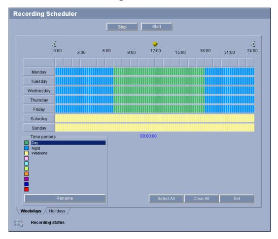
The recording scheduler allows you to link the created recording profiles with the days and times at which the images of selected cameras are to be recorded in the event of an alarm. You can link any number of 15-minute intervals with the recording profiles for each day of the week. Moving the mouse cursor over the table displays the time below it. This aids orientation.
