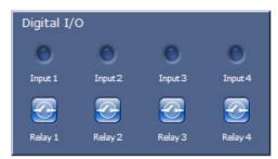
The alarm icons **Input 1** to **Input 4** are for information purposes and indicate the status of an alarm input: When an alarm is triggered, the corresponding icon lights up blue. The unit's configuration determines whether the alarm is displayed, as well as additional details (see *Section 5.15 Advanced Mode: LIVEPAGE Functions, page 43*).
