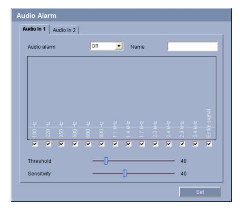
The VideoJet X40 can create alarms on the basis of audio signals. You can configure signal strengths and frequency ranges in such a way that false alarms, for example due to machine noise or background noise, are avoided.
