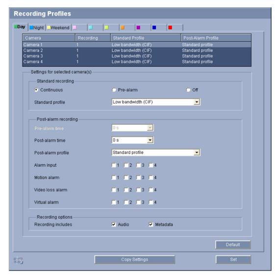
You can define up to ten different recording profiles. You will then use these recording profiles in the recording scheduler, where they are linked with the individual days and times (see Section 5.25 Advanced Mode: Recording Scheduler, page 59).
