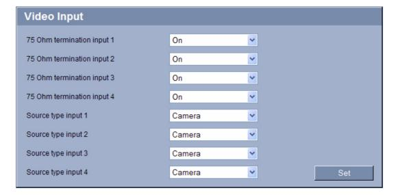
You can activate the 75 Ohm terminating resistance for each video input of the VideoJet X40. The terminating resistance must be deactivated for the video signal to be looped through. Every video input is closed at the time of delivery.
