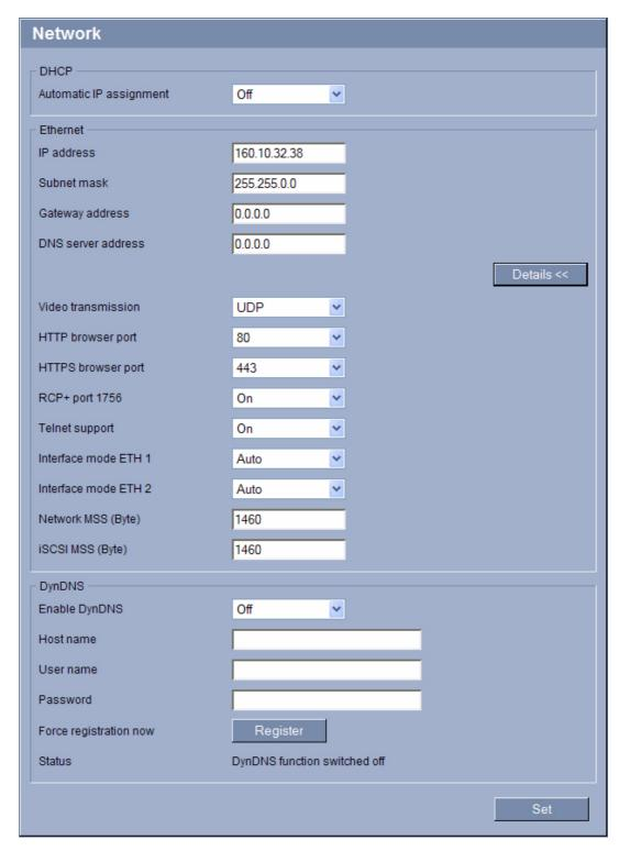
The settings on this page are used to integrate the VideoJet X40 into an existing network.
