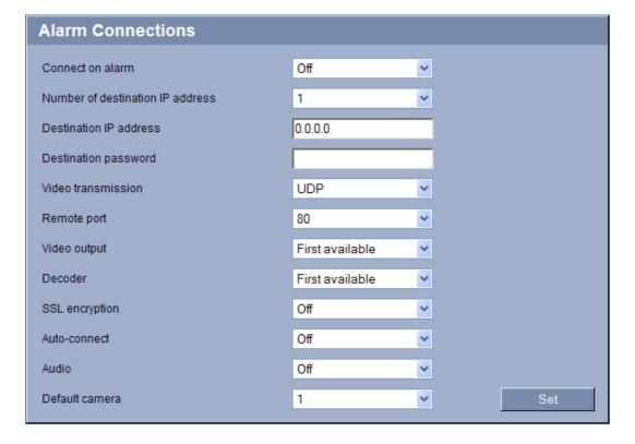
You can select how the VideoJet X40 responds to an alarm. In the event of an alarm, the unit can automatically connect to a pre-defined IP address. You can enter up to ten IP addresses to which the VideoJet X40 will connect in sequence in the event of an alarm, until a connection is made.
