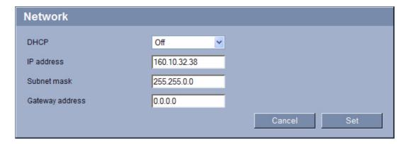
The settings on this page are used to integrate the VideoJet X40 into an existing network. Some changes only take effect after the unit is rebooted. In this case, the **Set** button changes to **Set and Reboot**.
