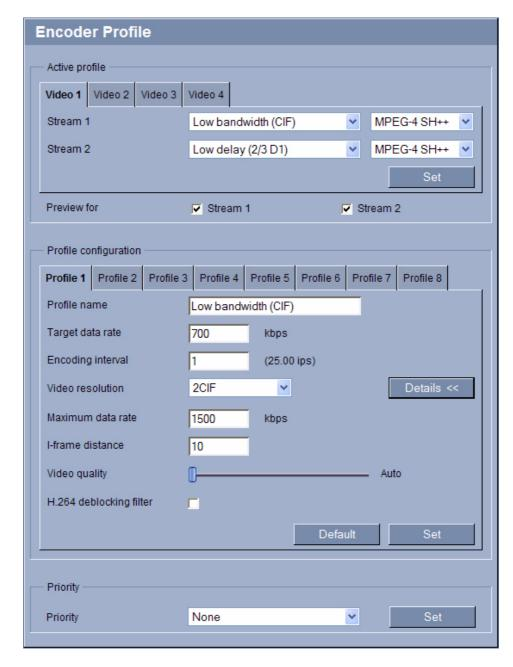
For the video signal encoding, you can select a code algorithm for each and two profiles for each encoder (video input), and you can change the presets for the profiles.
