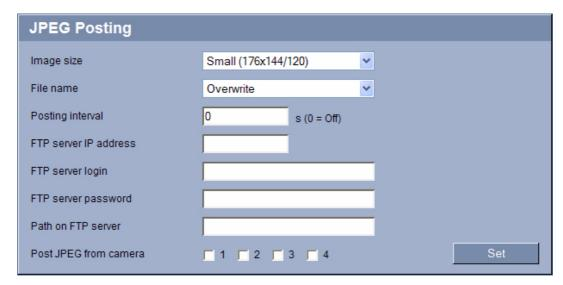
You can save individual JPEG images on an FTP server at specific intervals. You can then retrieve these images at a later date to reconstruct alarm events if required.
