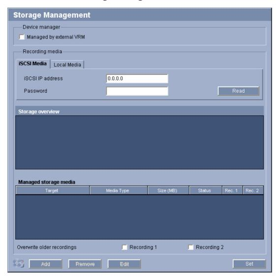
You can record the images from the cameras connected to the VideoJet X40 on various local storage media or on an appropriately configured iSCSI system.
