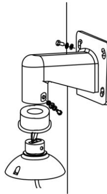
Wall Mounting: Pendant Mount (mounting example)
