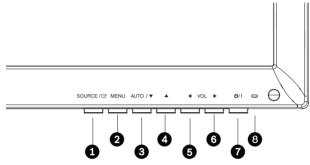
Figure 6.1 Front Panel Buttons
