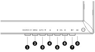
Figure 3.1 UML-193-90/UML-223-90 Front Panel
