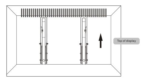
Adapter brackets should be pulled out to the extended position in order to install screws through proper holes.
