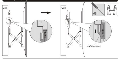
Hang top hook of adapter brackets onto the top wall plate rail. Push the safety clamps upward and tighten screws to secure the bracket.
