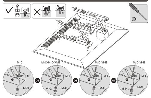
Note: Choose appropriate screws, washers and spacers (if necessary) according to the type of screen.
