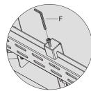
Slight adjustment allowed after display installation by loosening or tightening screws with an Allen key supplied.
