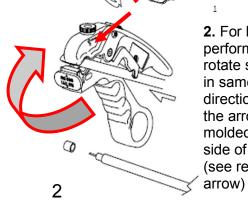
2. For best performance, rotate stripper in same direction as the arrow molded on side of tool (see red
