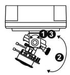
iii. Release the video adjustment screw and then adjust the lens direction. After completion, tighten the video adjustment screw.
