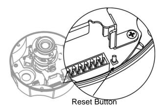
The Reset Button can be used to reboot the camera or restore it to factory default settings. If the camera experiences a problem, rebooting the camera may correct the problem. If the problem remains, please restore the camera to factory default settings and reinstall the software.
