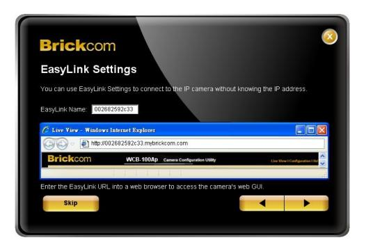
EasyLinkTM is a unique Brickcom function which allows users to assign a unique EasyLink name to their network camera's IP address. There is no need to configure the router to open up ports or remember hard-to-memorize IP addresses. Users can log onto [uniqueEasyLinkname].mybrickcom.com to view the camera's web GUI and live view.
