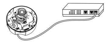
b. Connect the camera to a non-PoE hub via PoE Injector.
