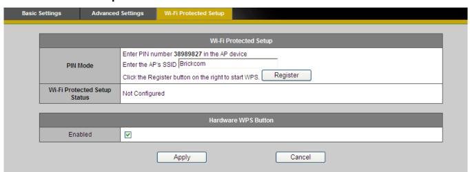
Use this method if the client device has a Wi-Fi Protected Setup PIN number.
