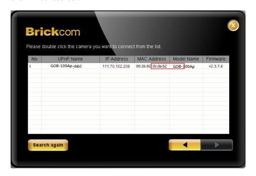
C. The network camera can now be accessed over a 3G network. To access the video feed through the internet, open a web browser and enter the network camera's IP address. A dialog window will pop up requesting a username and password. As stated on the previous page, the default username and password for the Administrator account are "admin/admin".
