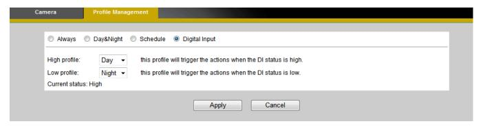
**Digital Inputs (\*)** (Only available with models with a DI terminal)- Select Digital Input to have the profile management controlled by an external sensor. Select profiles from the drop down menu. Profiles will change according to different trigger voltage levels.
