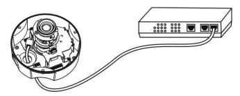
2) Connect the camera to a non-PoE hub via PoE Injector.
