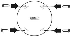
4) Mount the camera on the wall and position to four screw slots over the plastic anchors. Insert the screws into the holes and use the screwdriver to tighten the screws clockwise until they are secure.
