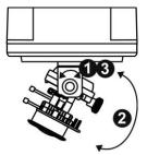
3) Release the video adjustment screw and then adjust the lens direction. After completion, tighten the video adjustment screw.
