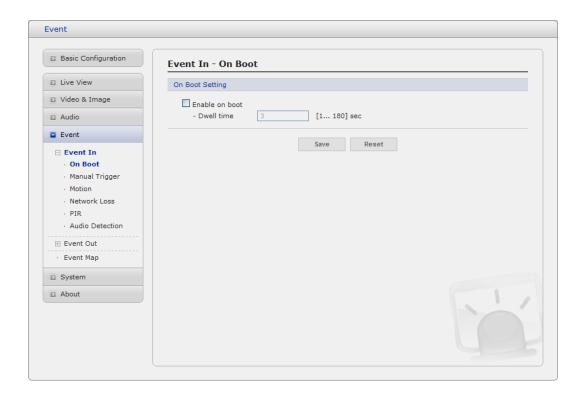
This is used to trigger the event every time the Network Camera is started. Select "Enable" to activate the motion event.
