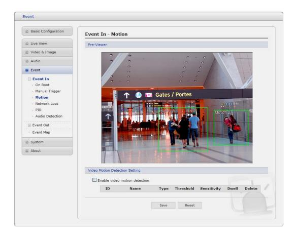
Motion detection is used to generate an alarm whenever movement occurs (or stops) in the video image. A total of 8 Motion and/or Mask windows can be created and configured.
