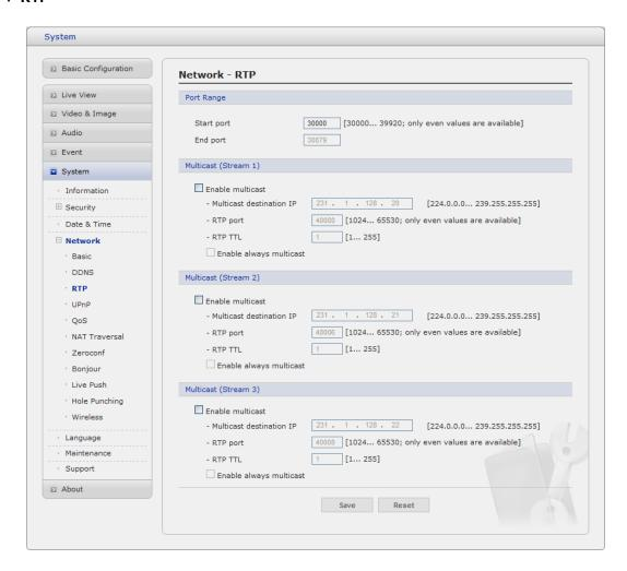
Have a setting for sending and receiving an audio or video on a real-time basis. These settings are the IP address, port number, and Time-To-Live value to use for the media stream(s) in multicast H.264 format. Only certain IP addresses and port numbers should be used for multicast streams. For more information, please see the online help.
