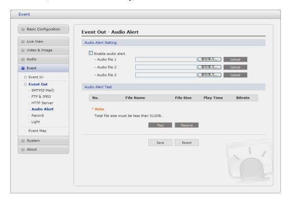
When the network camera detects an event, it can output a predefined audio data to external speaker. Check the box to enable the service.
