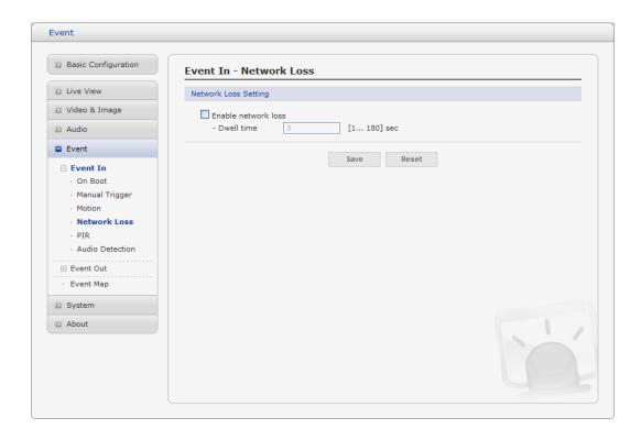
This is used to trigger the event every time the network connection is failed. Select "Enable" to activate the Network Loss event.
