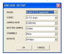
**Caution:** All parameters must be synchronized with ones in audio setting page of network devices for a proper operation.
