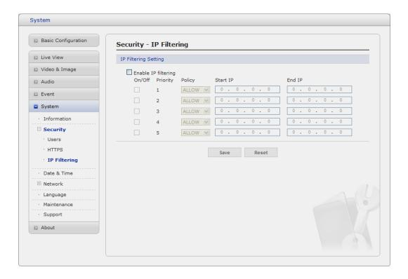
Checking the **Enable IP address filtering** box enables the IP address filtering function. Up to 256 IP address entries may be specified (a single entry can contain multiple IP addresses). Click the **Add** button to add new filtered addresses.
