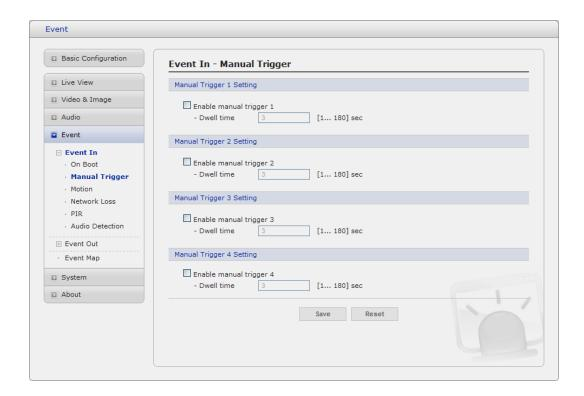
This option makes use of the manual trigger button provided on the live view page, which are used to start or stop the event type manually. Alternatively the event can be triggered via the product's API (Application Programming Interface).
