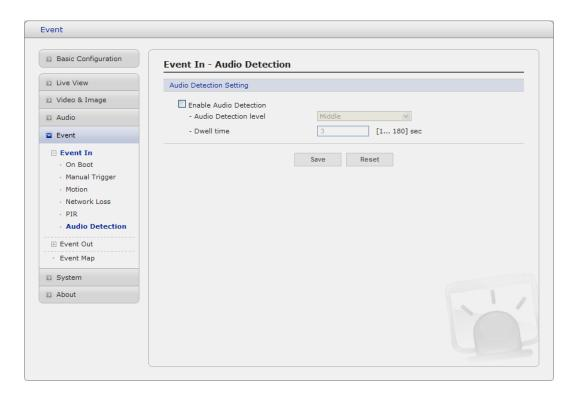
Audio detection can be used to measure change in the ambient voice.
