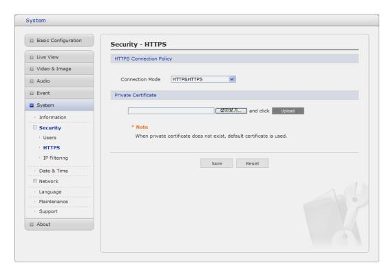
For greater security, the Network Camera can be configured to use HTTPS (Hypertext Transfer Protocol over SSL (Secure Socket Layer)). That is, all communication that would otherwise go via HTTP will instead go via an encrypted HTTPS connection.
