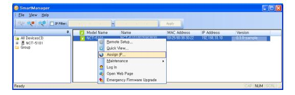
4. Select Assign IP. You cam see a Assign IP window. Enter the required IP address.
