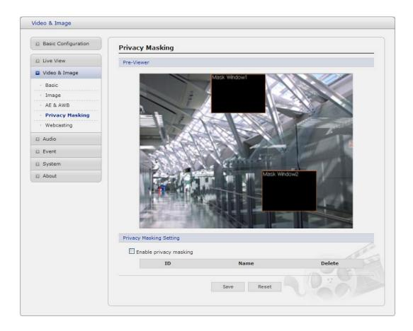
The privacy masks are configured by Mask windows. Each window can be selected by clicking with the mouse. It is also possible to **resize or delete**, **or move** the window, by selecting the appropriate window at the mouse menu on the video screen.
