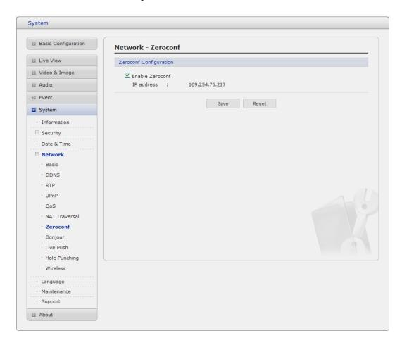
Zero configuration networking (zeroconf), is a set of techniques that automatically creates a usable Internet Protocol (IP) network without manual operator intervention or special configuration servers.
