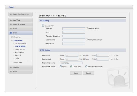
When the network camera detects an event, it can record and save images to an FTP server. Images can be sent as e-mail attachments. Check the box to enable the service.
