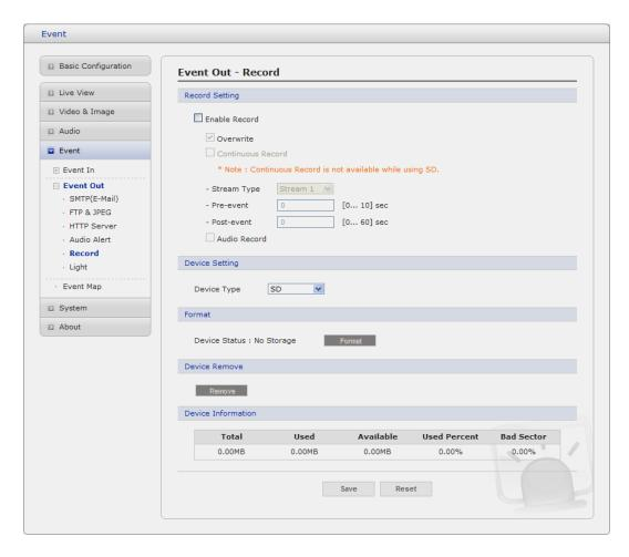
When the network camera detects an event, it can record video stream in the Micro SD Memory (not supplied) or NAS (Network Attached Device) as a storage device. Check the box to enable the service.
