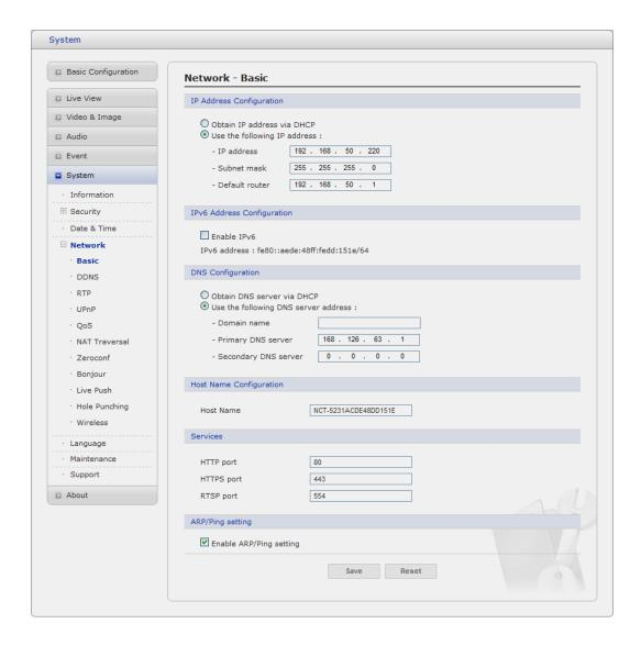
Setting in regard to network can be executed. Settings for IP, DNS, Host Name, Port, and ARP/Ping can be established, along with setting for DDNS, uPnP, QoS, Zeroconfig, Bonjour, Live Push, Hole Punching, and wireless.
