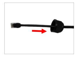
3. Insert the sealing insert with claw.
