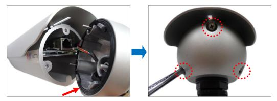
**CAUTION:** Make sure the rubber seal is properly attached and the back cover is closed to ensure water or dust cannot enter the camera.
