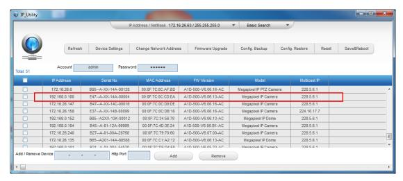
You can quickly see the camera model in the list. Click on the IP address to automatically launch the default browser of the PC with the IP address of the target camera filled in the address bar of the browser already.
