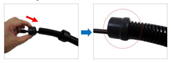
5. Insert the gland body into the Ethernet cable.
