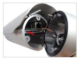
3. When done, ensure the rubber seal is aligned and attached to the back cover and then close the back cover by tightening the three (3) screws.
