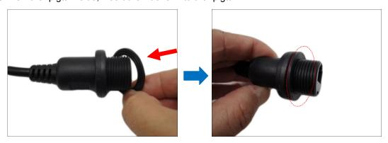
7. Connect the Ethernet cable connector to the "pigtail" connector.
