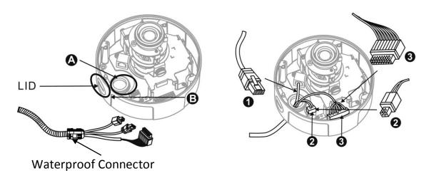
A compliant waterproof connector shall be attached tightly to the conduit hole of the Vandal Dome Network Camera, and all the cables shall run through the connector for the camera to be IP67-compliant.
