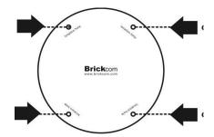
iii. Hammer the four plastic anchors which are provided in the product package into the four location holes. Mount the camera on the wall and position the four screw holes over the plastic anchors. Insert the screws into the holes and use the screwdriver to tighten the screws clockwise into the holes until they are fixed.
