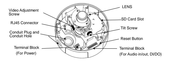
2. Below "Device Appearance Description" is for VD-100A-series/ VD-130A-series / VD-130N-series/ VD-300N-series/ VD-302N-seris/ VD-300A V3-series/ VD-302A-series/ VD-500A-series/ VD-502A-series
