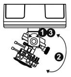
iii. Release the video adjustment screw and to adjust the lens direction. After completion, tighten the video adjustment screw.
