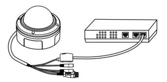
ii. Connect the camera to a non-PoE switch using the PoE Injector.
