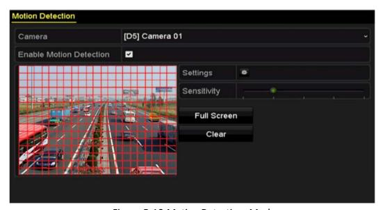
Figure 5-10 Motion Detection- Mask
