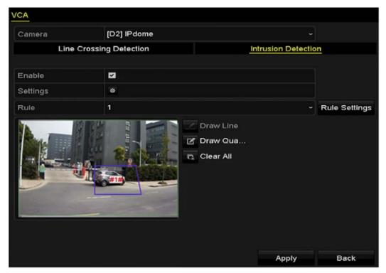
Figure 8-16 Draw Area for Intrusion Detection
