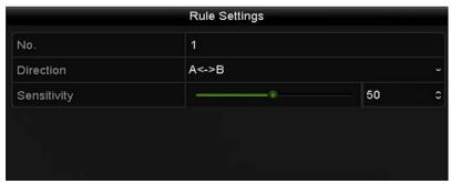
Figure 8-13 Set Line Crossing Detection Rules
