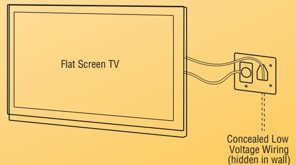
Use with either a single gang retrofit work box or a new nail on box for new construction.
