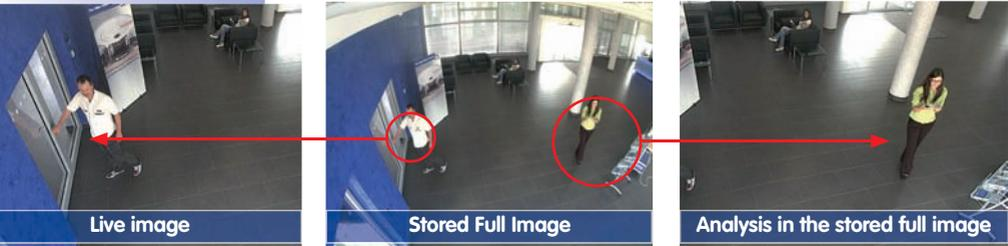
This means that you can use the vPTZ features in VGA resolution to pan, tilt and zoom the live image while the camera is e.g. recording full images at 1 fps in MEGA or QXGA resolution.
