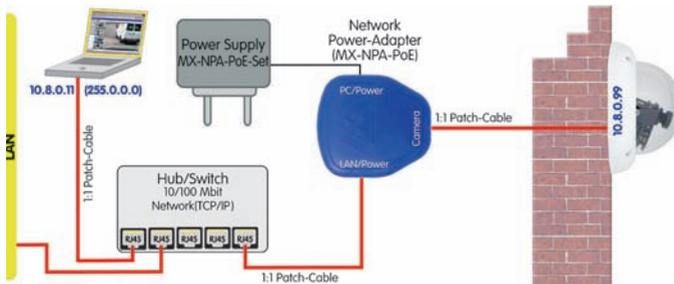
For the D24M, you should use the new blue MX-NPA-PoE-Set - previous MOBOTIX network power accessories such as the NPA Set, Power Box and Power Rack (MX-NPA-Set, MX-NPR-4 and MX-NPR8/20) are not suitable for use with the D24M
