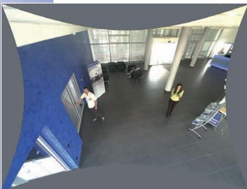
The image distortion caused by the L22 90° Wide Angle lens can be corrected (see Section 3.4). Since this function requires more computing power, it should not be enabled in the live image for applications that require a maximum frame rate. The image distortion in the recording can also be corrected at a later time.
