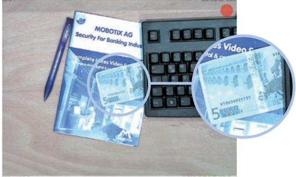
With a D24M equipped with an L22 lens, the (slightly) distorted image can be corrected by software (see Section 3.4)
