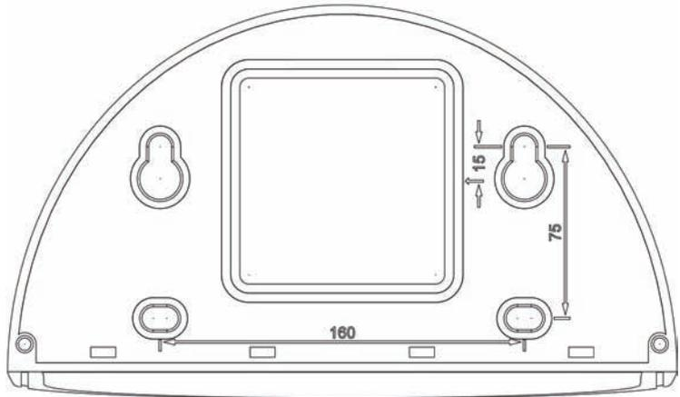
Direct installation over surface- and flush-mounted sockets
