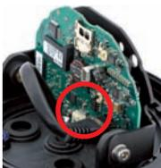
Push-push function: only remove the MicroSD card after first gently pushing it in
