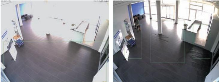
Placing the exposure window in the lower image area (left image) delivers less optimum results compared to moving three individual exposure windows up toward the windows (right image)
