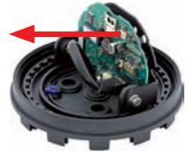
3. **Loosen the internal part of the camera** by releasing the two blue clamps with the thin side of the hook wrench.
