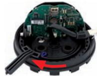
9. **Connect the network cable** to the network connector of the camera.
