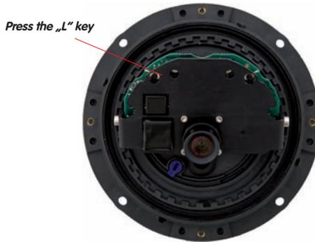
5. After about two more seconds, the camera is accessible via its factory IP address (see label on the camera housing).
