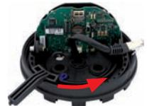
4. **Remove the internal part of the camera** with the lens mount from the base of the camera.
