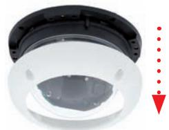
6. **Remove the mounting ring:** Separate the black mounting ring from the camera housing (lift the spring clip). This ring is not required when mounting the camera to the On-Wall Set.
