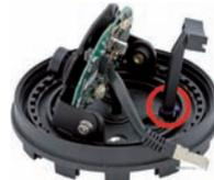
8. Now secure the internal part of the camera by turning the toothed ring in a clockwise direction until you can still turn the internal part of the camera without much force.
