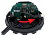
Loosen the ring and screws until you are still able to pan and rotate the internal part of the camera with the lens without much force but not so far that the lens is unable to move on its own.
