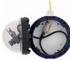
8. **Attach the camera to the mount:** Press the D24M so that it is seated firmly within the On-Wall Mount. The tapered guides at the back of the D24M housing fit exactly into the openings of the On-Wall Mount. Attach the white outer shell with the supplied Allen screws (without rubber seal) once the lens has been adjusted.
