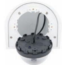
4. **Snap the camera into place on the bottom plate:** Firmly push the camera into the Wall Mount. The plastic spring clips will snap into place when the trapezoidal elements on the rear of the camera housing exactly match up with the corresponding openings on the Wall Mount.
