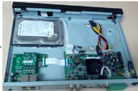
Place hard drive over screw holes and slide into place
