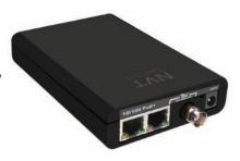
NV-PS56-60W: 56VDC power supply, 60 watts with IEC line cord
