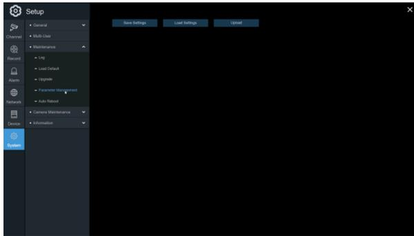
**Save Settings:** Click to save the NVR current system settings to the USB flash drive. Enter the Admin password to authenticate.
