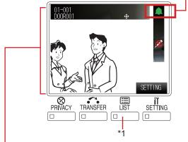
The station no., station name and video image at the calling station (following the station type image) are displayed.
