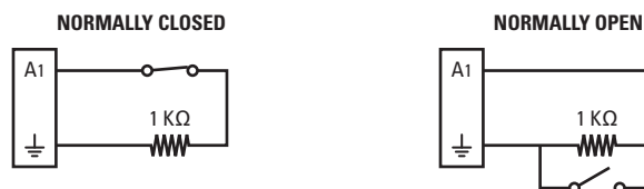
Figure 11. Supervised Alarm Input Wiring
