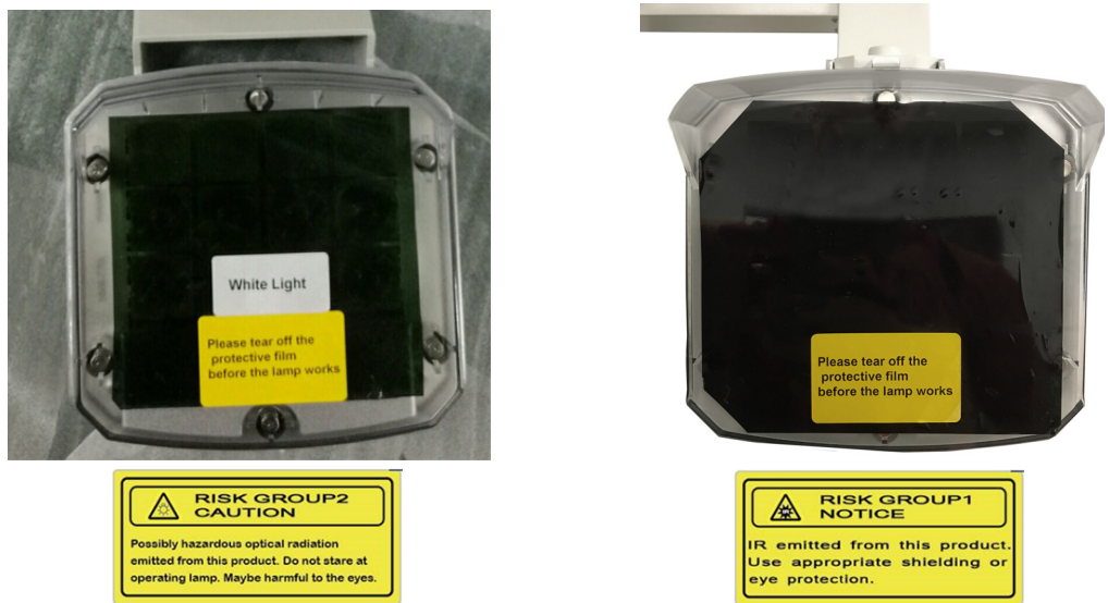
Figure 2. Protective Film Covering an White Illuminator (left), Protective Film Covering an IR Illuminator (right)
