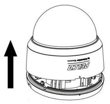
4. Replace by the new dome cover and click downward to complete the installation.
