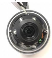
9. Adjust the angle of lens by pan and tilt by grasping the base.
