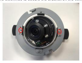
9. Adjust the angle of lens by pan and tilt. Grasp the base of the lens assembly to adjust.
