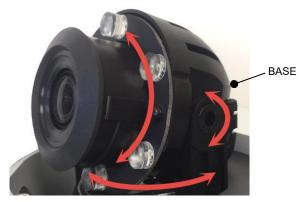
10. Tighten the locking screw to secure the camera module position.
