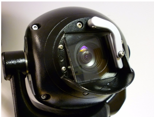
Figure 5.7 Inverted rain shield installed on camera
