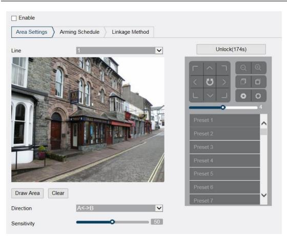
Figure 8-14 Line Crossing Detection
