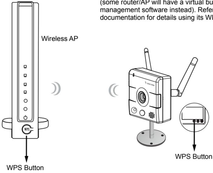
When WPS configuration is done, wireless connectivity will be established and the security encryption, such as WEP or WPA-PSK, will be synchronized with the AP. Use the IW2 utility to find the camera. As for IP setting, the camera's use of DHCP or static IP is determined by your configuration on the network camera via the web-based configuration of firmware. The camera's default is DHCP.
