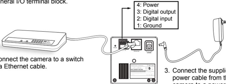
2. Connect the camera to a switch via Ethernet cable.
