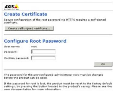
2. Enter a password and re-enter, to confirm the spelling. Click **OK**. If the password is lost, the camera must be reset to the factory default settings. See page 39.
