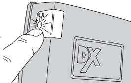
**AFTER PUSHING THE RECEIVER'S PROGRAMMING BUTTON, YOU ONLY HAVE 3 SECONDS TO SEND A SIGNAL BEFORE PROGRAMMING MODE STOPS**
