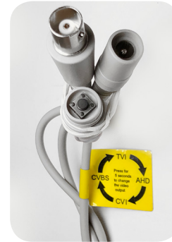
Field Selectable TVI/AHD/CVI/Analog with Dip Switch on Camera
