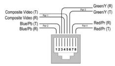
Plug one (1) balun into the component video coaxial cable output of the video source according to the color code of the RCA cable leads.
