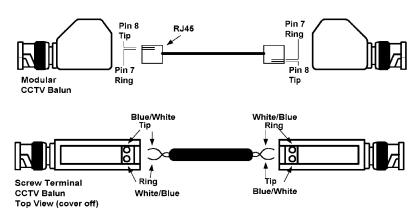
7. Power-on the CCTV equipment and check the picture quality. The video should be clear and sharp within the maximum specified distances. The following diagram shows a typical application.
