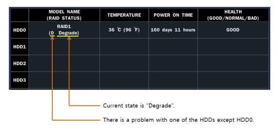
\*Open the top cover of the DVR and replace the HDD except HDD0 with a new one.
