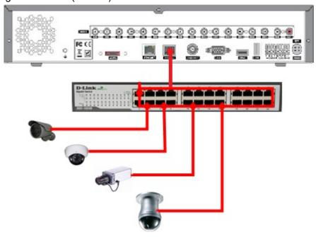
Figure 2.6.1.1. Proper connection example of the N32NS (Non PoE Switch).
