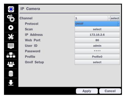
Figure 4.1.2 IP Camera Setup Screen (ONVIF)
