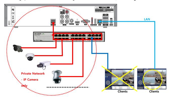
Figure 2.6.1.2. Improper connection of the N32NS
