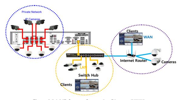
Figure 2.5.1.2 IP Camera Connection Diagram (N8NU)
