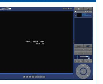
SpecoTech Multi-Client Viewer Software is a multiple site monitoring client software that allows streaming of video and audio, and transmission of alarm signals from the DVRs over the network. The SpecoTech Multi-Client can display up to 16 DVRs and supports dual monitors. PTZ camera control is also supported by this software.
