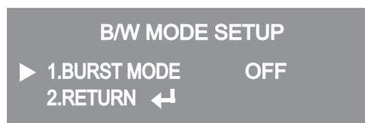
◆ **AUTO** : The mode is switched to 'Color' in a normal environment, but switches to 'B/W' mode when ambient illumination is low. To set up the switching time for AUTO mode, press the Function Setup switch. You can turn on or off the burst signal on B/W mode.
