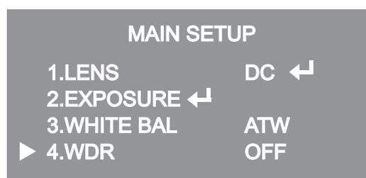
1. When the SETUP menu screen is displayed, select 'WDR' by using the switch so that the arrow indicates 'WDR'.
