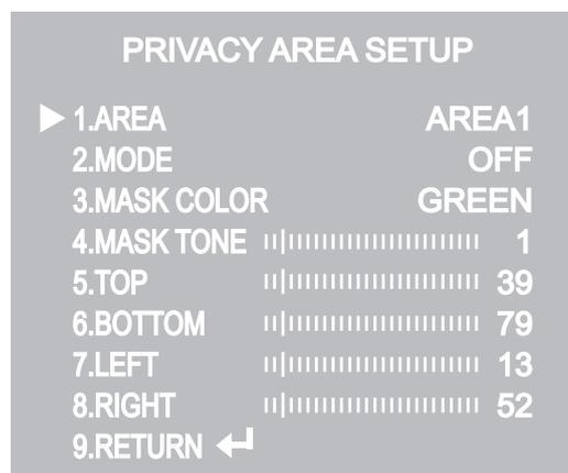
1) When the SPECIAL menu screen is displayed, press the Function Setup switch so that the arrow indicates 'PRIVACY'.
