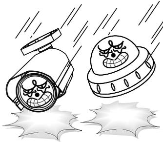
Housing damage can compromise weatherproof ratings.
