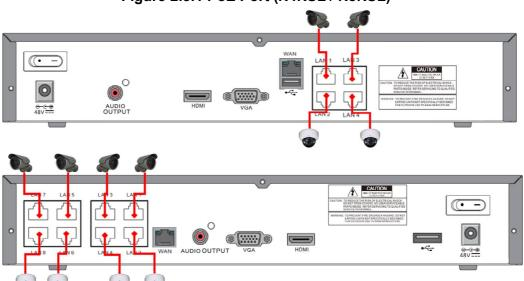
Figure 2.5.1.1 IP Camera Connection Diagram (N4NSL, N8NSL)
