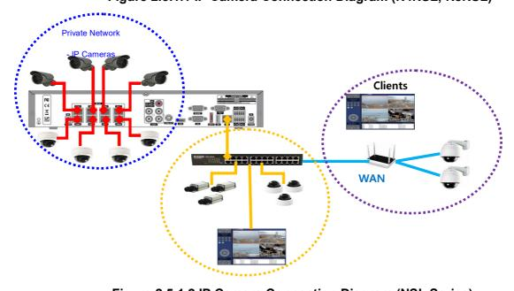
Figure 2.5.1.2 IP Camera Connection Diagram (NSL Series)
