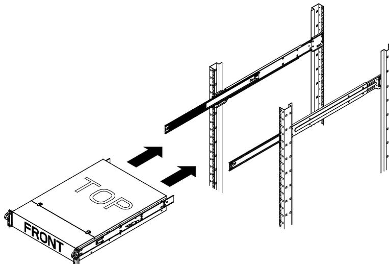
**To install the chassis in the rack:**
